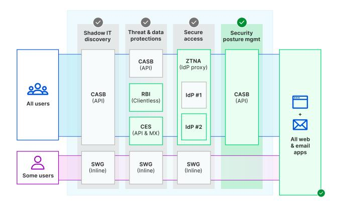
SWG = secure web gateway | CASB = cloud access security broker | IdP = identity provider | RBI = remote browser isolation CES = cloud email security | ZTNA = Zero Trust network access
