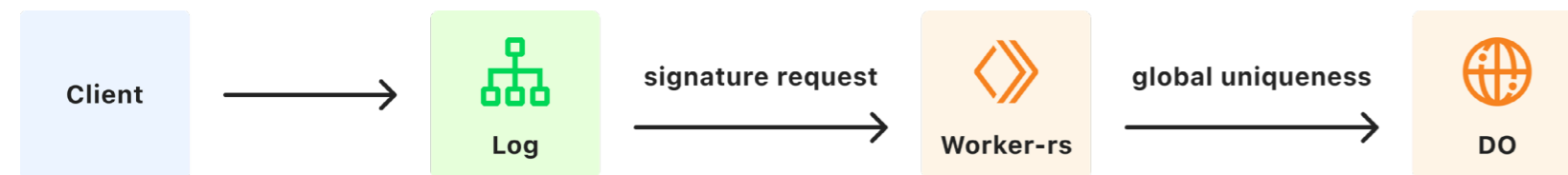
⚡ Timestamping service architecture (Cloudflare Workers in Rust, using a Durable Object for storage).
